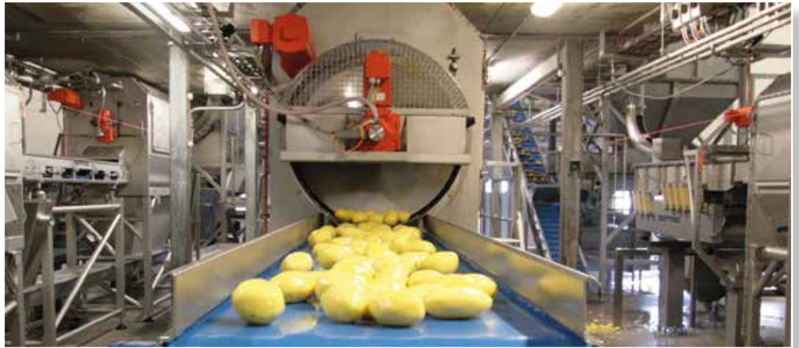
Knife peeled potatoes coming from the MS knife peeler. The product looks smooth as hand-peeled with avoiding of flat peeling.
