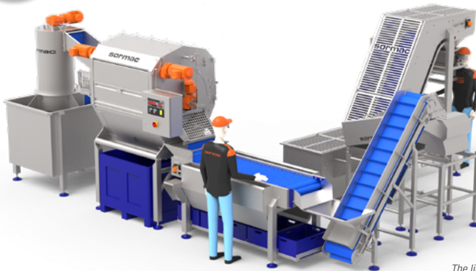
The line as shown processes potatoes up to 900 kg/h. Machines from left to right: screw destoner - knife peeler - roller inspection table - transport conveyor - sliver remover - weighing machine.
