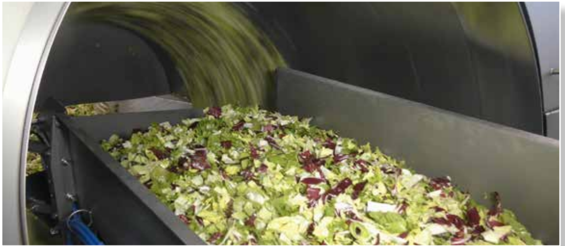
A special designed cross conveyor provides a unique way of filling the drum and prevents damage to the product.
