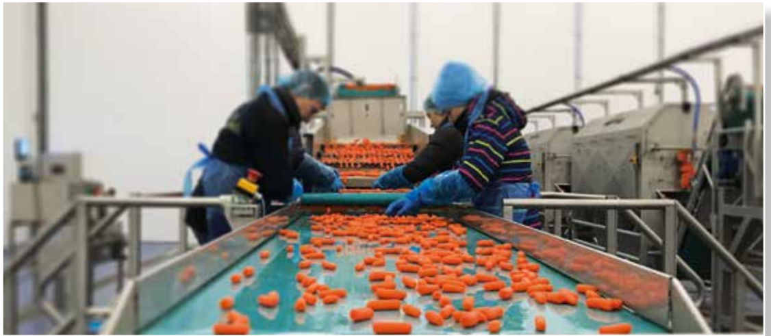
Baby carrots are manually inspected after being polished in the revolver peelers. Optionally, carrots can be inspected by an optical sorter. After inspection, the product core temperature is cooled down in a hydrocooler.
